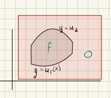
This region is called y-simple, the other is called x-simple. Simple means either, and appears to be the same as elementary.
